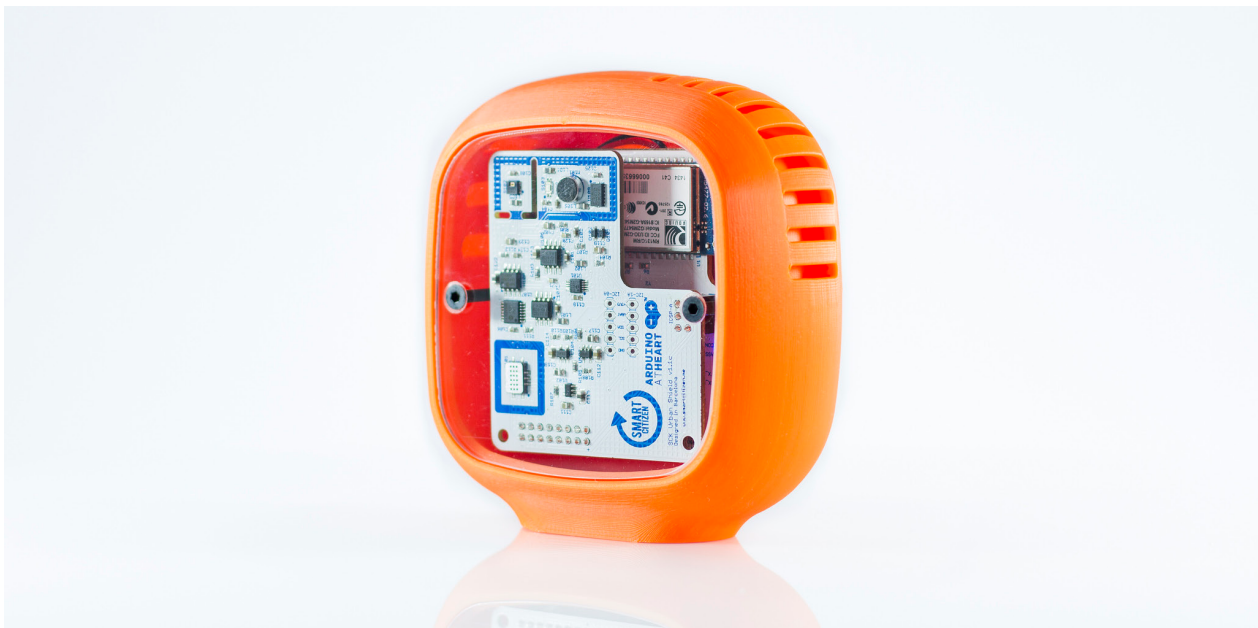
Fig 18 The Smart Citizen Kit 1.1 with the 3D Printed enclosure
