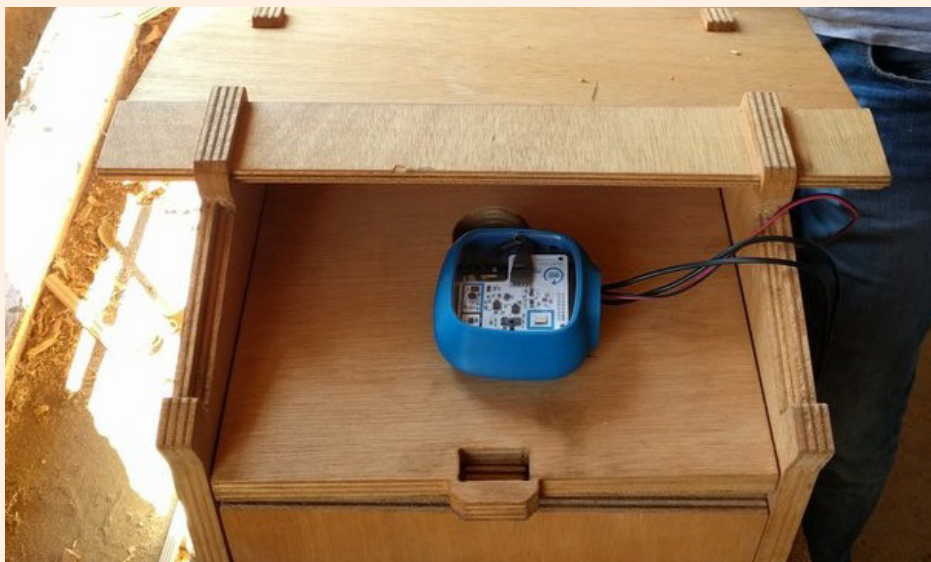
Fig 21 The Smart Citizen Kit expanded for the Open Source Beehives team being set on a Beehive at the Green Fab Lab
